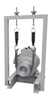
ASC A-ET26 DC Compound Motor Lab is an exclusive training system designed for Electrical Machine lab to demonstrate the operation of DC compound motor. With this training system we can understand the fundamental operating principle of DC Compound Motor. This product includes various experiments such as No Load Test, Load Test and Operating Characteristics of DC Compound Motor.
